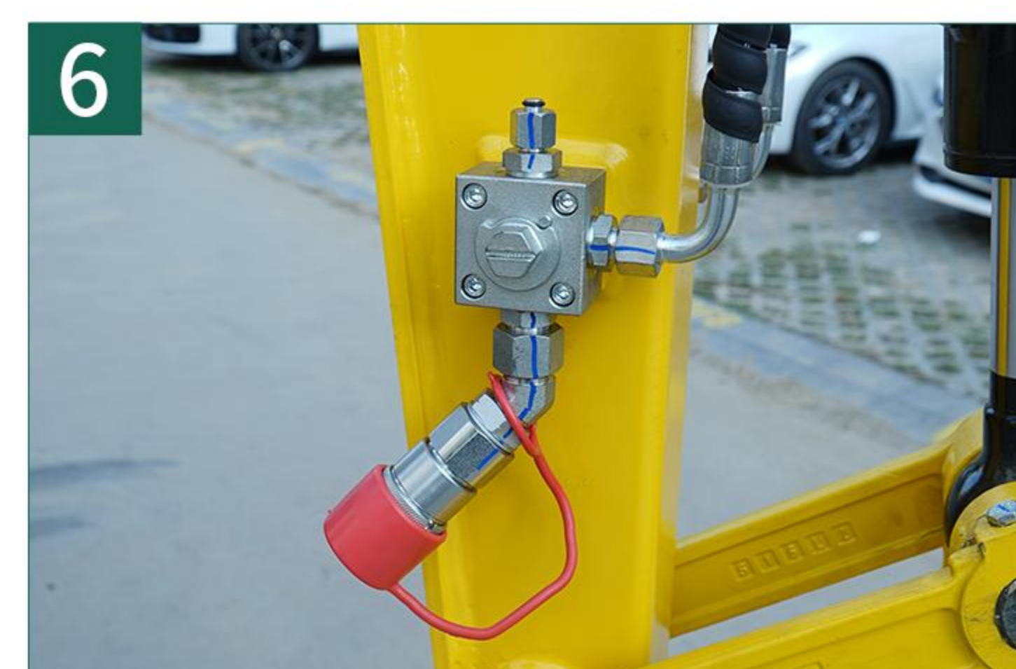
Crushing hammer shut-off valve
